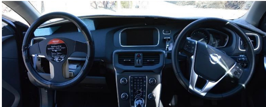
Figure 4.6: AVIP prototype interior. Fake steering wheel on the left, real steering wheel on the right. Reprinted from [49]
