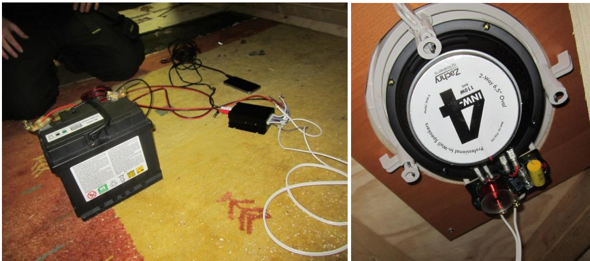
Figure 46 Connecting the speakers to the car battery
