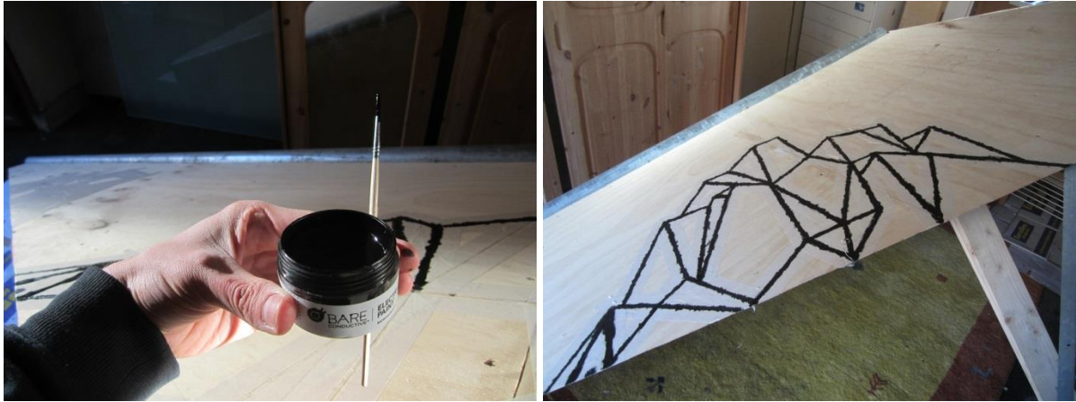
Figure 45 Painting the prototype with conductive paint
