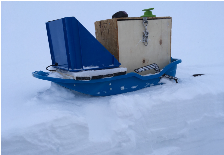
Figure 4.1: The complete radar system implemented on a sled.
