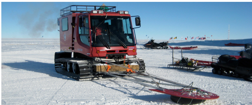
Figure 1.1: Image of a typical GPR mounted on a snow groomer. From [2]
