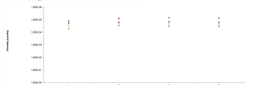
Figure 3: Average intensity of each compound in standard mix + blood spot for all ESI needle positions tested, negative ionization mode.
