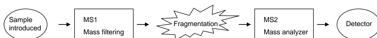
Figure 3 Illustration of tandem MS. Tandem MS is when the MS analysis includes mass filtering and fragmentation before detection.
