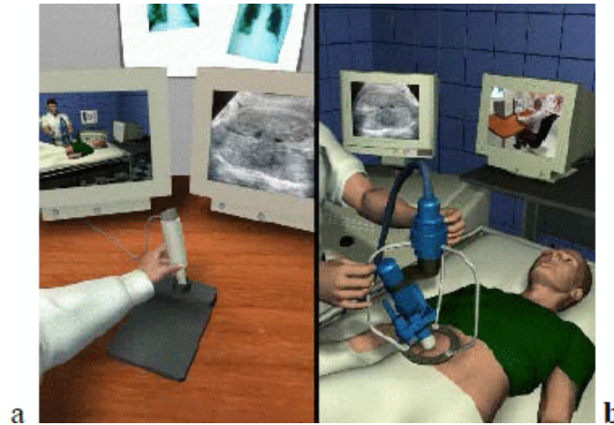
Figure 2.1: A graphical render of the ESTELE system as seen from the controller (a), and patients (b) perspective [10]
