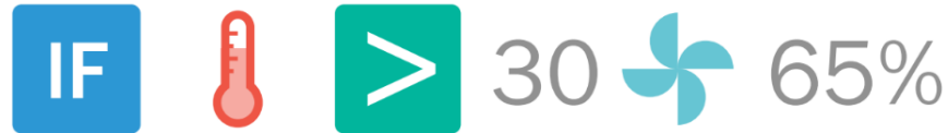
Figure 1.1: If the temperature is above 30 units, turn on the fan at 65% power. The unit was not specified by the creator. Credit: Jon Bøhmer.
