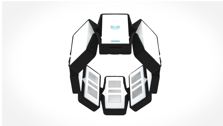
Figure 2.4: Myo sensor armband. The band contains 8 EMG sensors, a gyroscope, an accelerometer and a magnetometer. [19]
