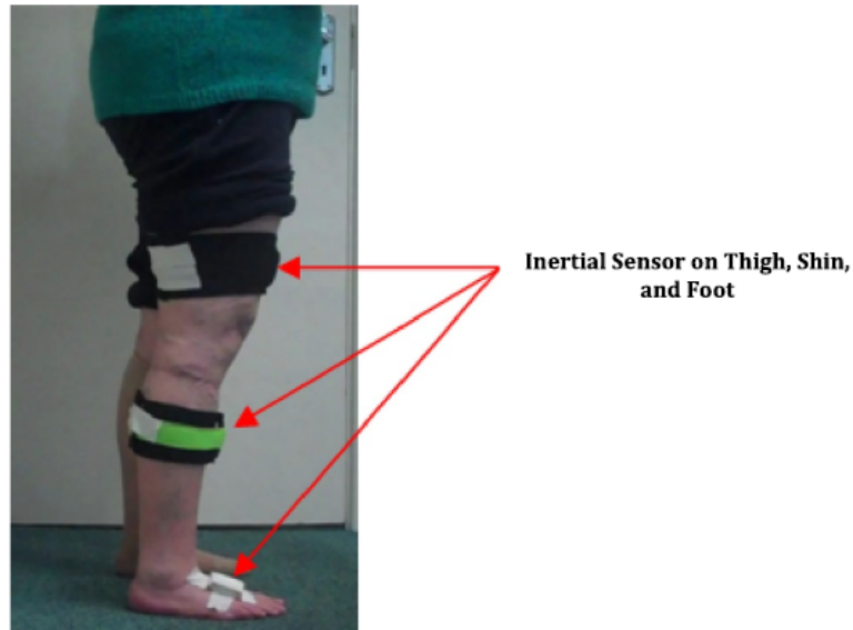
Figure 2.13: Sensors attached to the right light for orthopedic exercise evaluation in [11]
