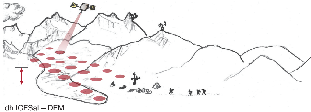
Figure 1.2: Elevation differences ( dh ) between ICESat footprints and a reference DEM on a mountain glacier.
