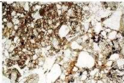
Fig. 4: Photomicrograph of M14073C (C16012), layer 10090a; compact soil and burned sandstone rock forming levelling layer. PPL, frame width is ~30mm.
