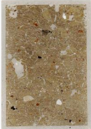
Fig. 1: Scan of M107B (Layers 3/4, S107), showing crack/fissured structure, burrow mixed pale subsoil, more humic soil and iron mottling. Frame width is ~50mm.
