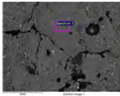
Fig. 27: X-ray Backscatter image of clayey intercalation in M8 (see Fig 24); note surrounding silty soil.
