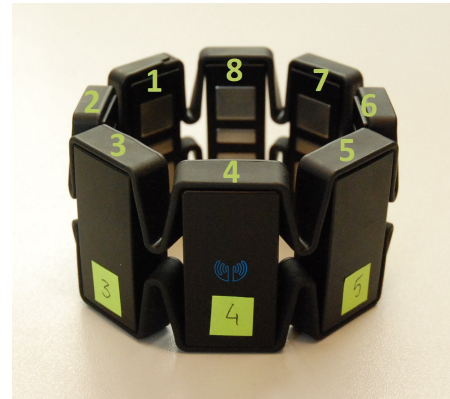
Figure 1: The Myo armband with the sensor numbering according to Thalmic Labs.
