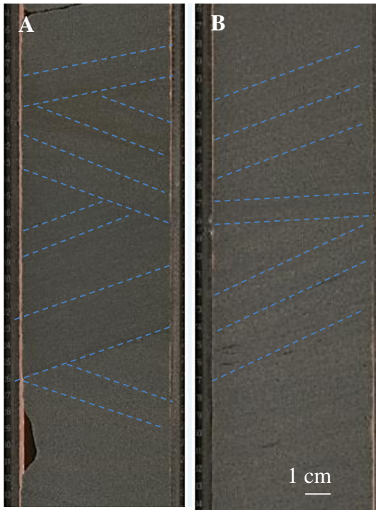
Figure 18: Pictures from the interval 1368-1369m (A) and from 1380-1382m (B). The higher mud content (A) compared to the lower part of the core makes them more visible.
