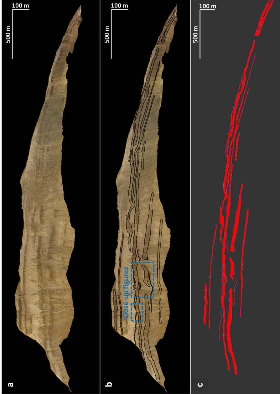
Figure 5.1: 3D view of the entire virtual outcrop model of El Manzano in raw form (a) and with interpreted sill complex (black lines, b). A section through the resulting model is shown in (c) with red and dark areas representing sills and host rock, respectively. The images are vertically exaggerated by a factor of 2. Blue squares indicate locations of close-up views shown in figure 5.2.
