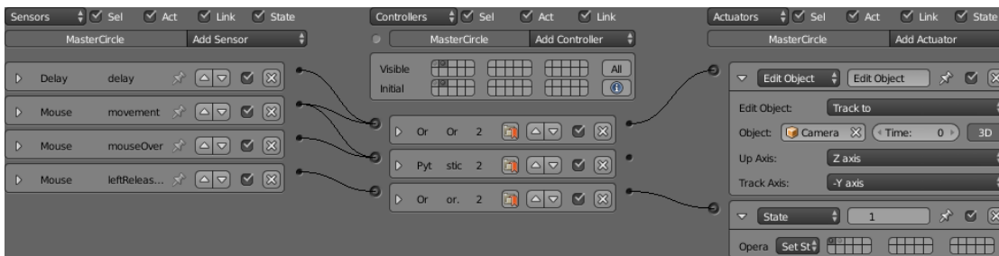
(c) Logic for state 2. With the mouse button still pressed, a Python script is called, which makes the object follow the mouse pointer.
