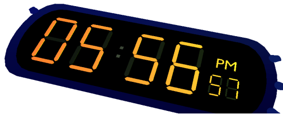
Figure 11.3: As the original watch, when the light is turned on it becomes harder to differentiate between active and inactive segments.
