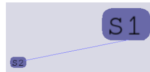
Figure 10.12: OpenGL's internal lines do not honour perspective.
