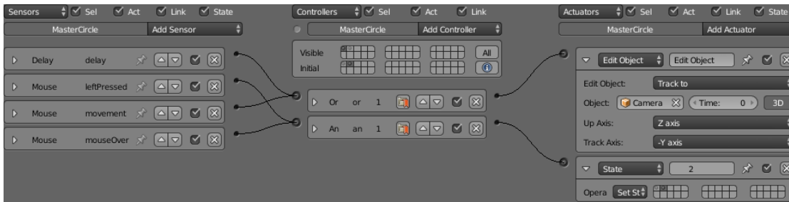
(b) Logic for state 1. While it awaits a click on the object to switch to state 2, it billboards to the camera.
