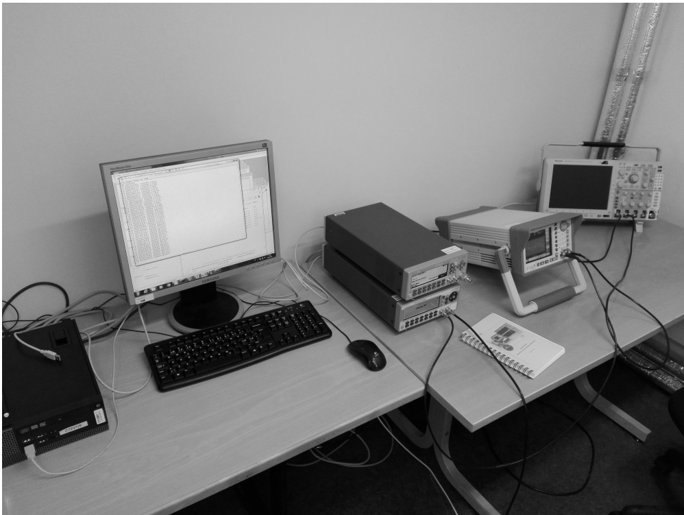
Figure G.1: Photograph of the system used to measure the 10 MHz output from the atomic clock. Not in the picture is the source of the 10 MHz reference.
