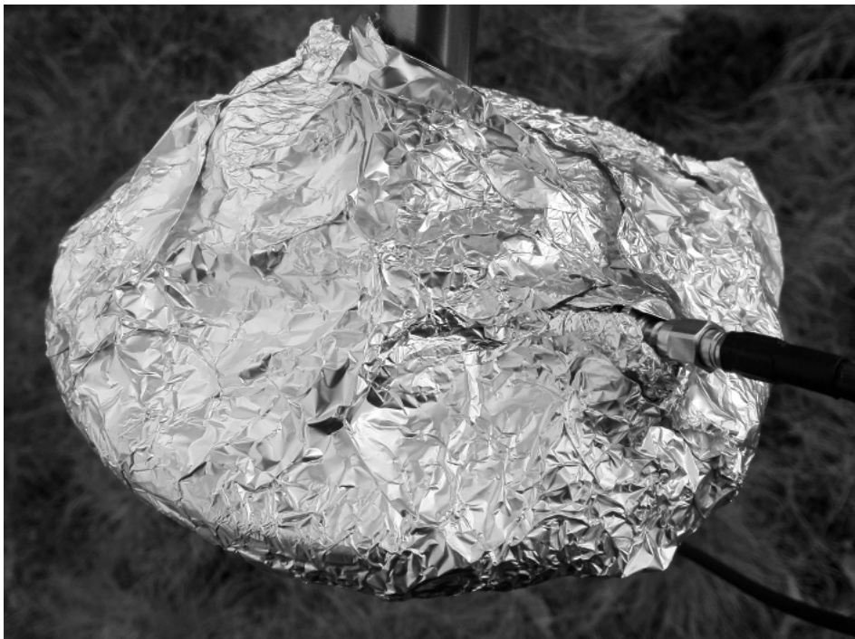
Figure G.2: Antenna covered in aluminium foil to simulate a jamming attack.
