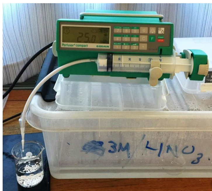
Figure 14: Custom experimental setup used in this work. A syringe pump pumps MOF/alginate mixture at a rate of 25 mL per minute. Pipette tips with four different diameters are connected to the PVA hose. Free fall distance was ~4 cm.
