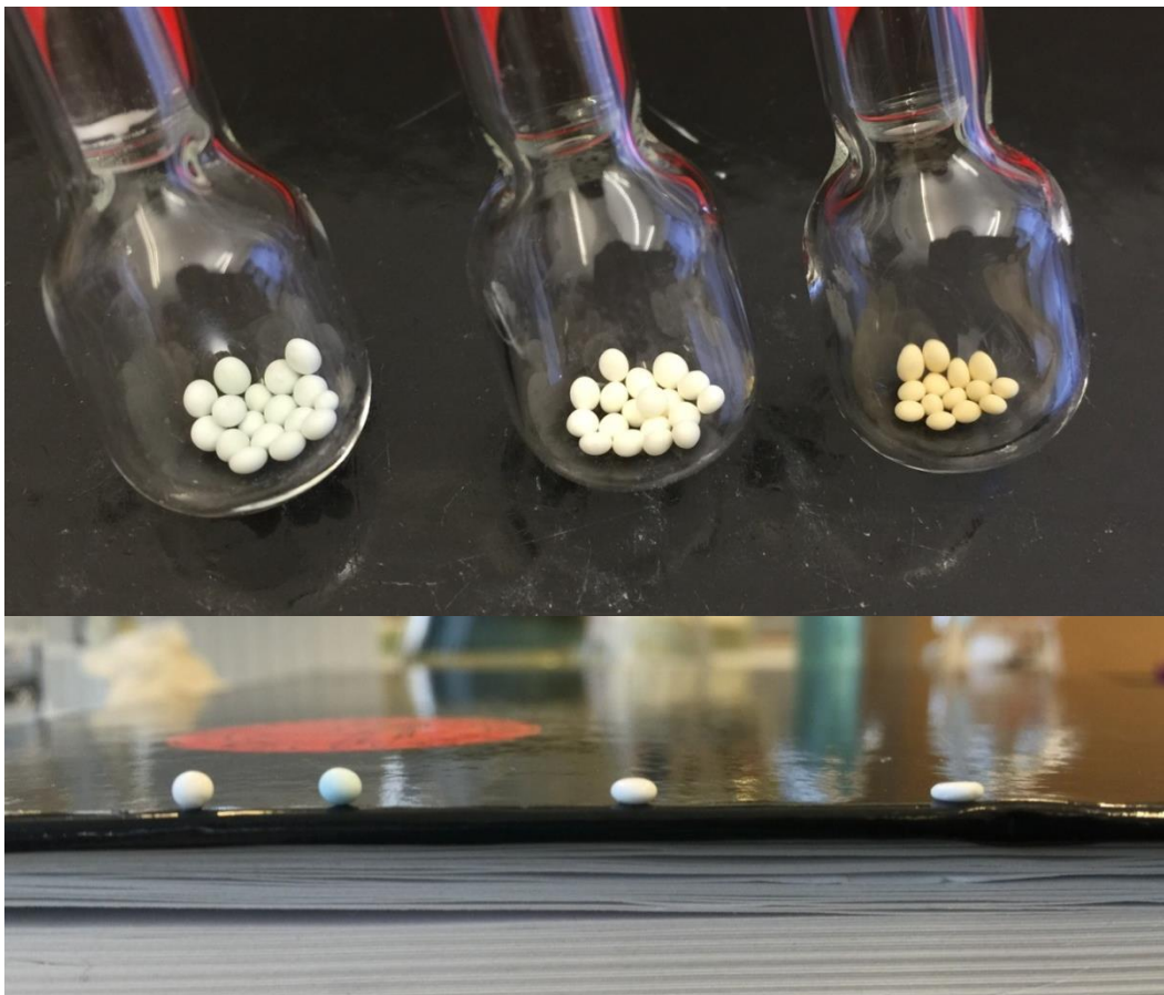
Figure 53: Top, from left to right: Cu-beads, Al-beads and Zr-beads. After activation at 120 °C for 2 hours under vacuum. Bottom, from left to right: Ca-bead, Cu-bead, Al-bead and Zr-bead. Right after gelation.
