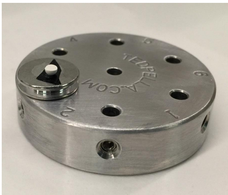
Figure 22: MOF bead sample preparation. A bead cut in half placed on a disk plate using a carbon tape (black).
