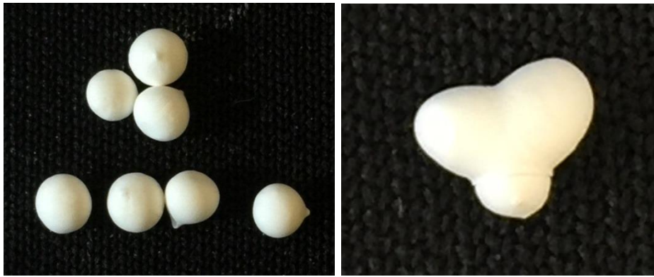
Figure 36 Tear-shaped beads of DWL-9-Ca10.0% (left). Three beads clung to each other (right).
