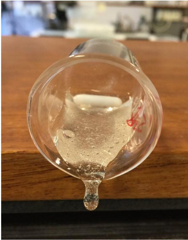
Figure 62: Highly viscous alginate solution due to high alginate concentration makes it harder to produce MOF-beads
