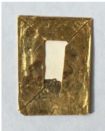
Figure 24: Sample prepared for FTIR measurement. Crushed and pressed MOF pellet inside a golden envelope.
