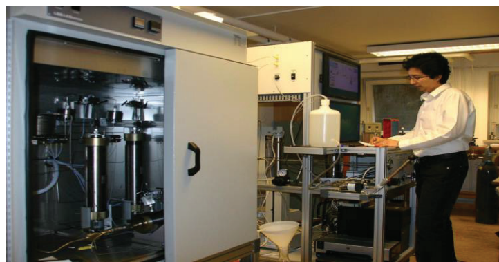
Figure 2: AFS-200 Core-Lab HP-HT flooding system
