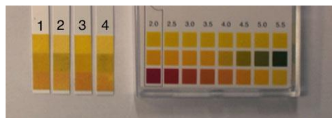
pH-indikatorstrips etter rensing
