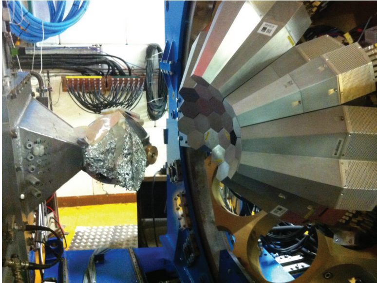
Figure 5.2: The \gamma photons were detected in 19 crystals from the AGATA \gamma tracking Ge array, positioned 23.5 cm from the target chamber.
