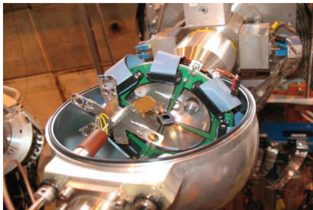
Figure 3.4: The annular Double Sided Silicon Strip Detector (DSSSD), mounted inside the MINIBALL target chamber for the ^{140}\text{Sm} Coulomb excitation experiment. The target wheel allows mounting of several targets in one experiment.
