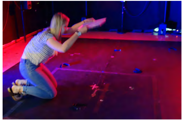
Figure 2. Calibrating the 20 AX3 sensors, by moving all of them rapidly up and down in a synchronization routine.
