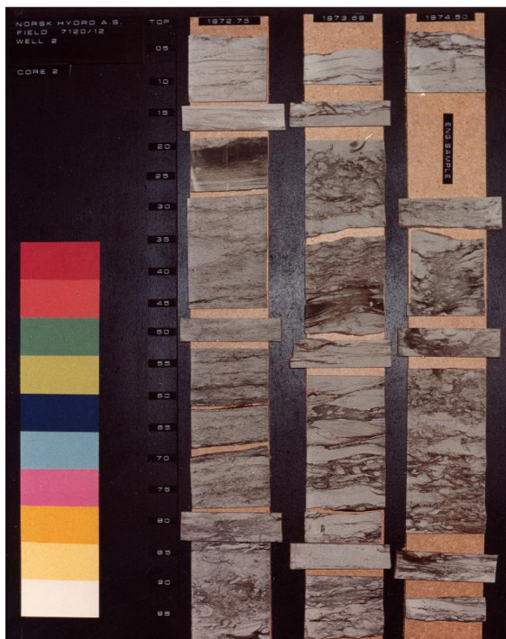
Figure 7-2. Argillaceous sandstone with frequent shale laminations in the interval of Stø formation in well 7120/12-2, corresponding to unit 2B. Depth: 1783-1786 MBSF. From NPD factpages (factpages.npd.no)
