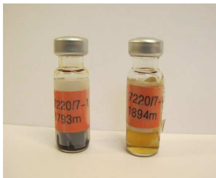
Figure 3.5: Oil from the Johan Castberg field, well 7220/7-1. The samples are taken from 1793m and 1894m. Both samples are diluted with dichloromethane (DCM).
