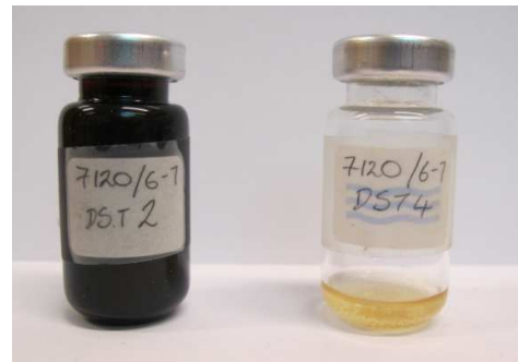
Figure 3.8: Oil (S1) and condensate (S2) from the well 7120/6-1. The oil is taken from 2432.05-2436.02 m and the condensate is taken from 2386.00- 2401.00m.
