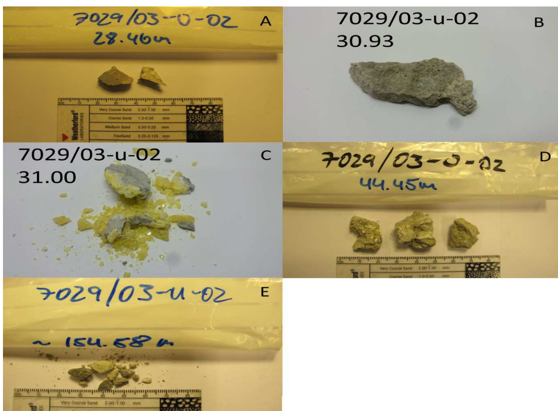
Figure 3.10: The Figures are shallow cores from the Finnmark Platform. The core 3.9A is taken from 28.46m, 3.9B is taken from depth 30.93m, 3.9C are taken from 31.00m below the sea bed, the fourth core sample Figure 3.9D from depth 44.45m and the last sample (Figure 3.9E) is taken from 154.58m below the sea bed. The 3.9C sample has a very high amount of sulfur.
