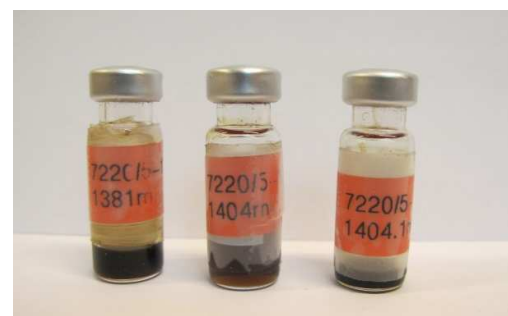
Figure 3.4: Oil from the Johan Castberg field, well 7220/5-1. The samples are taken from 1381m, 1404m and 1404.1m. The sample taken from 1404m is diluted.
