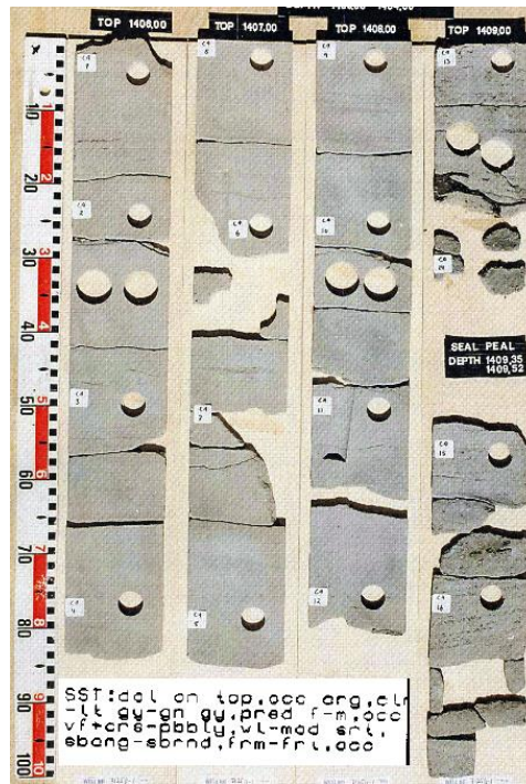
Figure 5.24. Core photo of the Stø Formation sandstone in well 7125/1-1, from depth 1406-1409 m. Description from the drilling company is included along the bottom. Modified from NPD (2015b).
