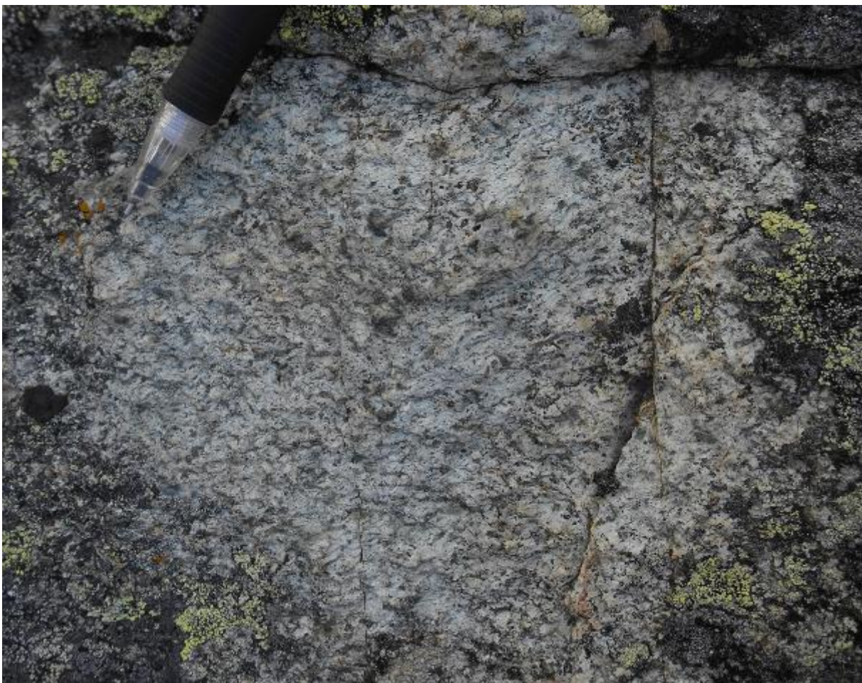
Figure 4.17: Texture in the intermediate intrusion. Note the light colour and dark mineral grains. This is a weekly foliated version.
