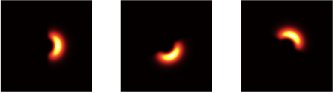
Figure 4.3: Fourier specter of the quadrature filters with center frequency \omega = \pi * 2^{-2} , bandwidth b\omega = 1 and direction n_1 = [1, 0]^T , n_2 = [\frac{1}{2}, -\frac{\sqrt{3}}{2}]^T and n_3 = [\frac{1}{2}, \frac{\sqrt{3}}{2}]^T . The Fourier domain is shifted so that the zero frequency is in the center of the image.
