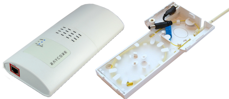
Figure 3.16: Raycore RC-OE2ATR - The media converter used.
