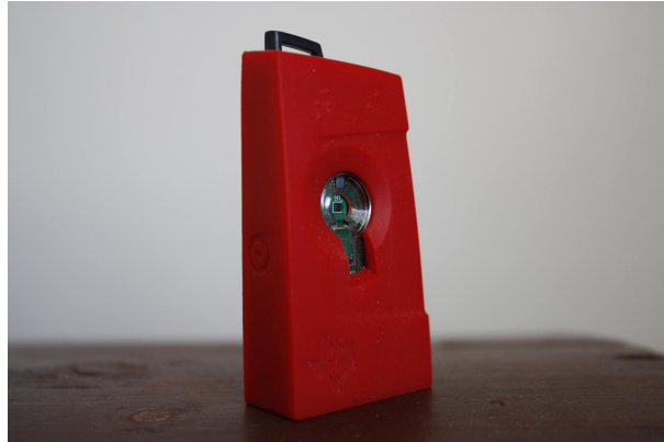
Figure 5.2: One of the TI SensorTag CC2541 Bluetooth beacons used in this thesis
