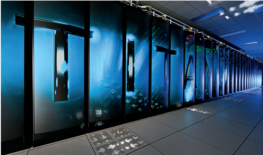
Figure 1: The Titan supercomputer consists of 18688 compute nodes and was used in connection with Paper IV. The total compute capacity of the machine is 27 Petaflops. Image courtesy of Oak Ridge National Laboratory.
