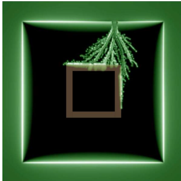
FIG. 1. Numerical simulation of the flux distribution in a superconducting film, where the propagation of an avalanche was blocked by a metal frame (light-brown). The brightness of the green color represents the magnitude of the flux density.
