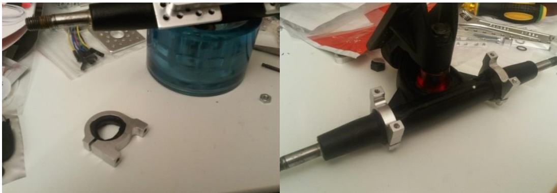
Figure 8.5 Clamp filled with Sugru before attaching (left), and trucks with both clamps attached (right)
