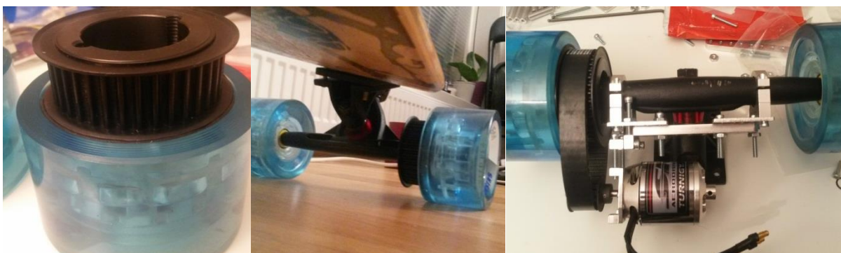
Figure 8.4 Timing pulley attached to wheel (left, middle), and first iteration motor mount (right)
