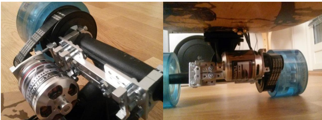
Figure 8.13 First iteration motor mount and transmission
