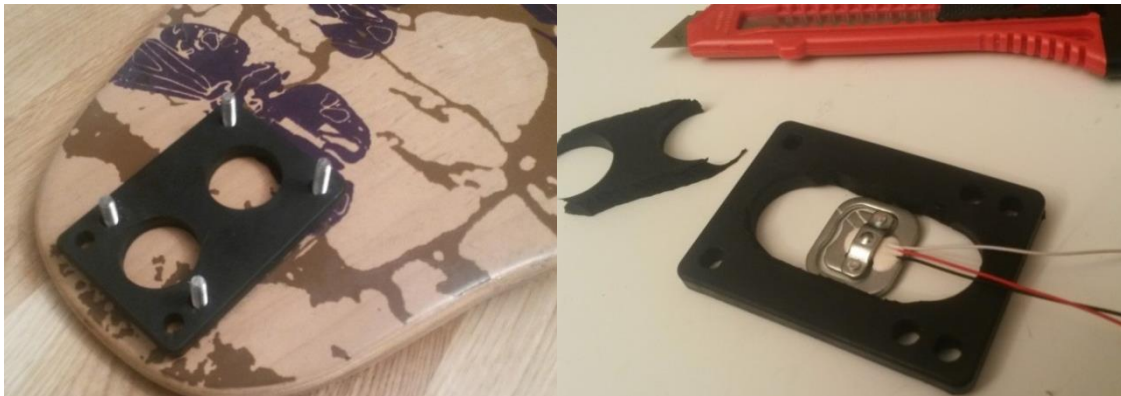
Figure 8.7 Risers on the board before cutting (left), and after cutting riser to fit the load sensor inside (right)
