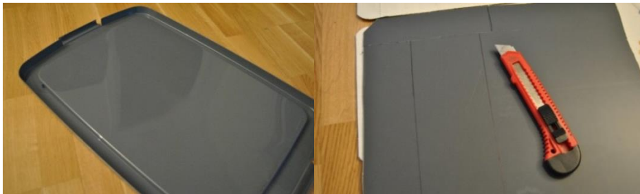
Figure 8.19 Cutting a plastic casing for the prototype electronics
