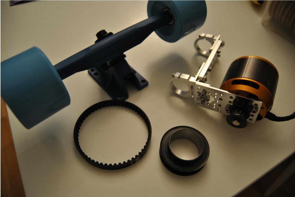
Figure 14.16 Prototype #2 drive-train components
