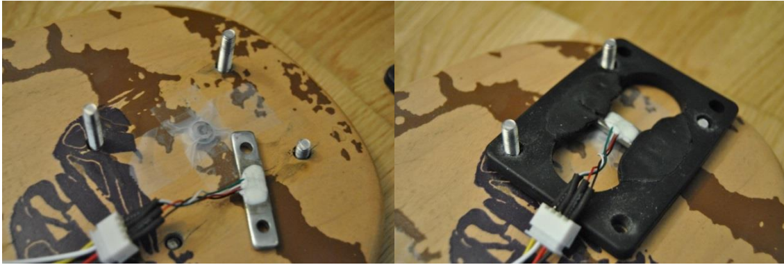
Figure 8.10 Close-up of bump and load cell before installation (left). Installed sensor inside the truck riser (right)
