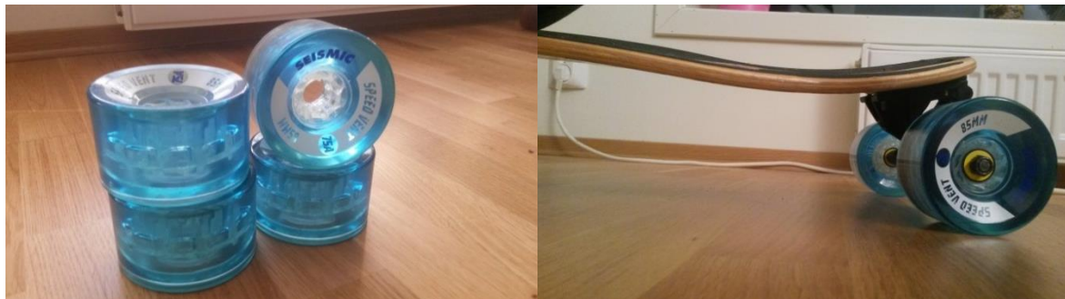
Figure 8.2 The 85mm wheels used on the prototype
