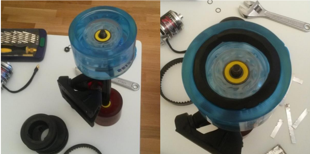
Figure 8.3 The wheel on vertically standing truck (left). Close-up of the wheel after attaching Sugru (right).
