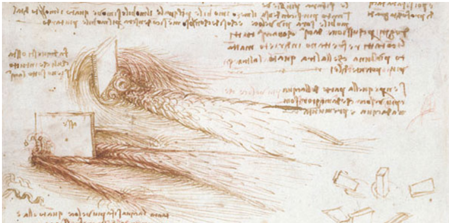
Figure 1.1: A rigid obstacle in flowing water, as sketched by Leonardo da Vinci in 1508-1509 (Nature).
