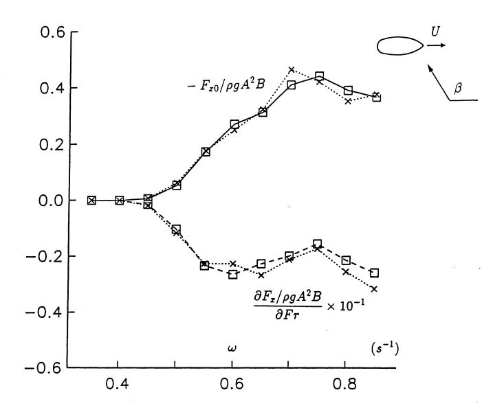
Figure 1: Mean drift force  $F_{x0}$  at zero forward speed (solid line) and wave drift damping coefficient  $\partial F_x/\partial Fr$  (dashed line) vs. wave frequency  $\omega$  of the incoming waves. Incidence angle  $\beta = 160^{\circ}$ . Dotted lines:  $F_{x0}$  and  $\partial F_x/\partial Fr$  for  $\beta = 180^{\circ}$  (head waves).  $\partial F_x/\partial Fr$  is obtained by numerical differentiation of  $F_x$  computed for  $Fr = \pm 0.02$ .
