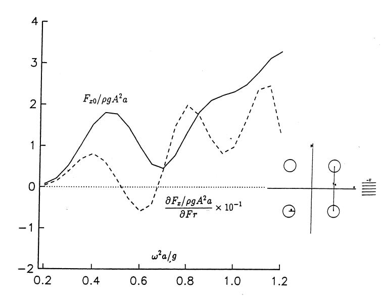
Figure 7: Mean drift force  $F_{x0}$  (solid line) and wave drift damping coefficient  $\partial F_x/\partial Fr$  (dashed line) for an offshore platform vs. wave number of the incoming waves. Incoming head waves. Platform free to surge in linear motions.  $\partial F_x/\partial Fr$  is obtained by numerical differentiation of  $F_x$  computed for  $Fr = \pm 0.005$ . (Nossen, Grue and Palm 1991).
