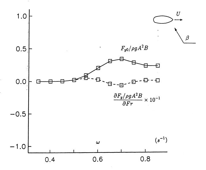
Figure 3: Lateral component of the mean drift force  $F_{y0}$  at zero forward speed (solid line) and  $\partial F_y/\partial Fr$  (dashed line) vs. wave frequency  $\omega$  of the incoming waves. Incidence angle  $\beta = 160^{\circ}$ .  $\partial F_y/\partial Fr$  is obtained by numerical differentiation of  $F_y$  computed for  $Fr = \pm 0.02$ .
