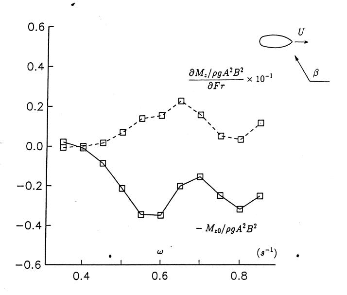
Figure 5: Mean yaw moment  $M_{z0}$  at zero forward speed (solid line) and  $\partial M_z/\partial Fr$  (dashed line) vs. wave frequency  $\omega$  of the incoming waves. Incidence angle  $\beta = 160^{\circ}$ .  $\partial M_z/\partial Fr$  is obtained by numerical differentiation of  $M_z$  computed for  $Fr = \pm 0.02$ .
