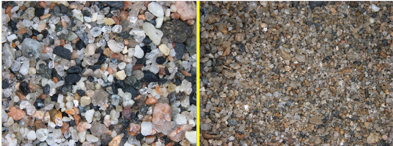
Figure 3-2 Illustration of grain size at Huk (a) and Nettet (b), both pictures were taken of the same magnification of 7.5 times by means of LM-Nikon SMZ.
