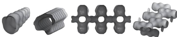
Fig. 7 Illustration of the pore system in a) TON b) MTT c) MWW and d) EUO zeolites.
