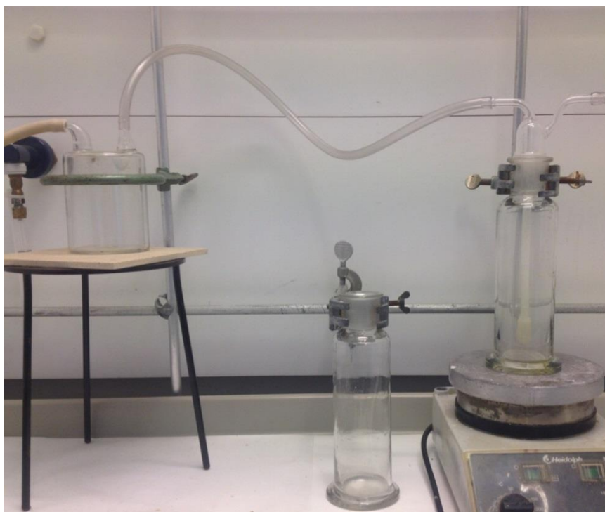
Figure 10: Experimental setup for the neutralization of mother liquor by ammonia gas. The beige tube entering the picture through the left frame was connected to the gas bottle. It is connected to a water-trap which was intended to collect any liquid which might migrate against the intended direction of gas flow. To the left is the gas-washing bottle wherein the mother liquor was contacted with the ammonia. The gas-washing bottle is mounted on a magnetic stirrer. The tube leaving through the right frame of picture leads any effluent gas directly to the fume-hood exhaust vent. In the center of the picture is a bottle used for holding the head of the gas-washing bottle whenever the gas flow was not on.
