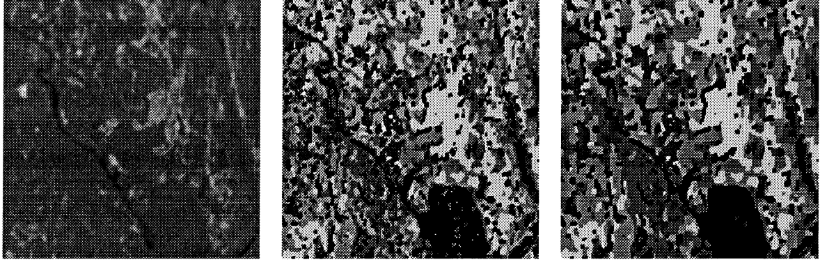
Figure 6: To the left, a texture image computed at Norwegian Computing Center based on a SAR image from ESA/EURIMMGE/TSS/Spacetex. The grey levels correspond to values in the range from 0 (black) to 255 (white). In the middle, the solutions obtained by ICM and to the right, the solution obtained by LR3. The classes are water, urban areas, forest, agricultural fields (unplowed) and agricultural fields (plowed), displayed from dark to bright.
