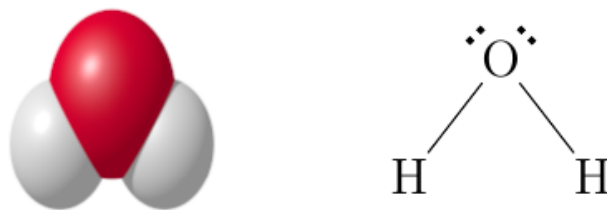
Figure 3.3: Illustration of a water molecule in molecular dynamics. The red sphere is the oxygen with its point charge and the two white spheres are hydrogens. They are in a distance r = 1.0 \text{ \AA} from the oxygen atom. The angle spanned by the two vertices' (covalent bonds) is \theta = 109.47^\circ
