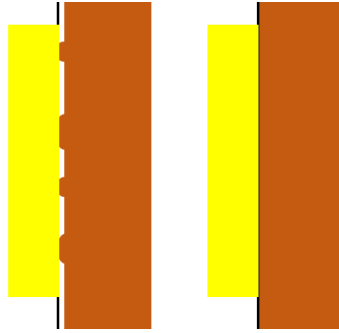
Fig. 4.9 (right) sensor resting on a few sand grains and (left) sensor in full contact with the sample
