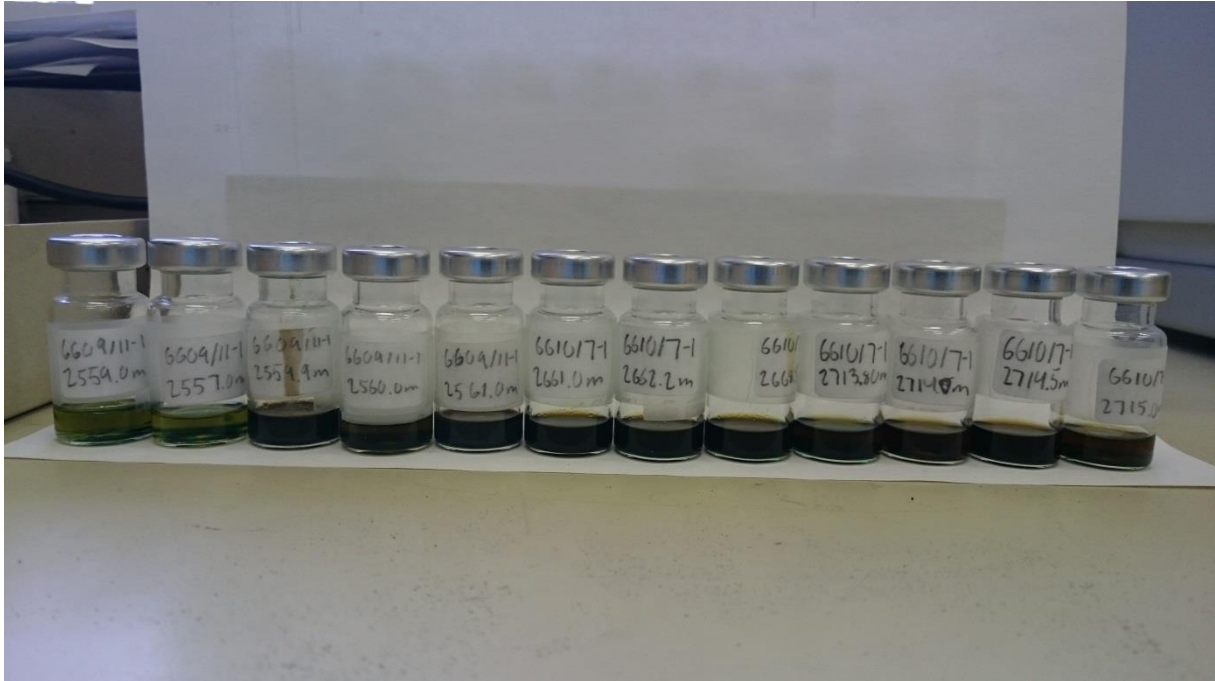
Figure 3.5: Extracted bitumen samples from sandstones in the dry wells 6609/11-1 and 6610/7-1 in the Helgeland Basin. As observed are most of the core extracts very dark in colour and this reflect usually a rich organic extract. The extracts were made using a Soxtec apparatus and the extraction media was DCM and MeOH (93:7 vol) (see section 4.2, Analytical Methods).
