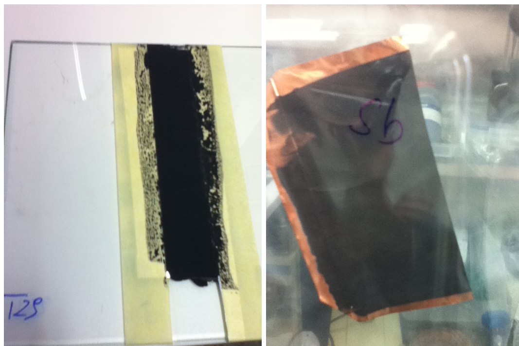
Figure 3.2: Left: Anode made of a - P/C tape T29, Right: Anode made of FeSb_2
