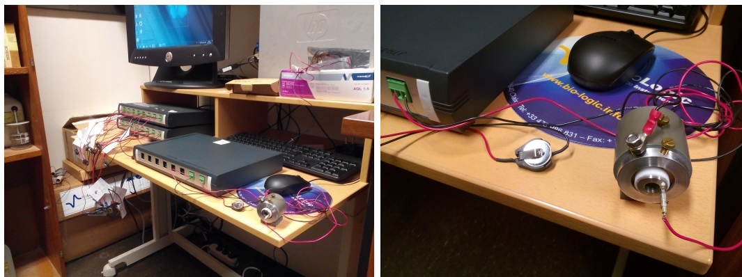
Figure 3.6: Left: BattSMALL galvanostat connected to a computer in the laboratory; Right: Our electrochemical cell and a coin cell in a holder for the operando measurement
