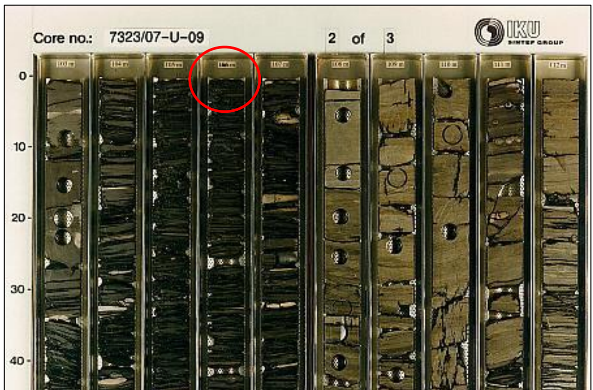
Figure 6: IKU stratigraphic drilling core photograph for the shallow core 7323/7-U-9 for the interval between 103.00-113.00 m. Mark the depth 106.00 m encircled in red that provided sample "S10" ( www.sintef.no )
