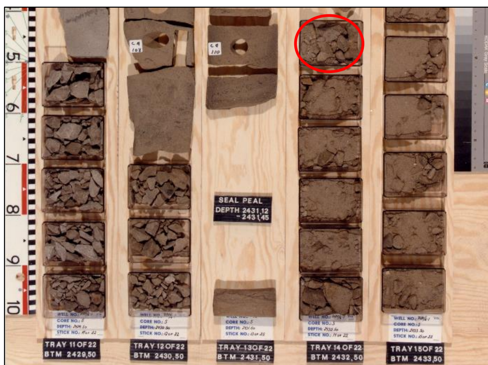
Figure 1: Core photograph for Well 7120/6-1 for the interval between 2428.50-2433.50 m. Mark the depth 2432.0 m encircled in red from where sample "E1" was recovered (Norsk Hydro, www.npd.no )
