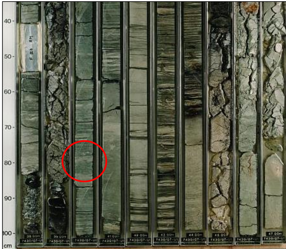
Figure 7: IKU stratigraphic drilling core photograph for the shallow core 7430/7-U-1 for the interval between 37.00-47.00 m. Mark the depth 38.80 m encircled in red that provided sample "S11" ( www.sintef.no )
