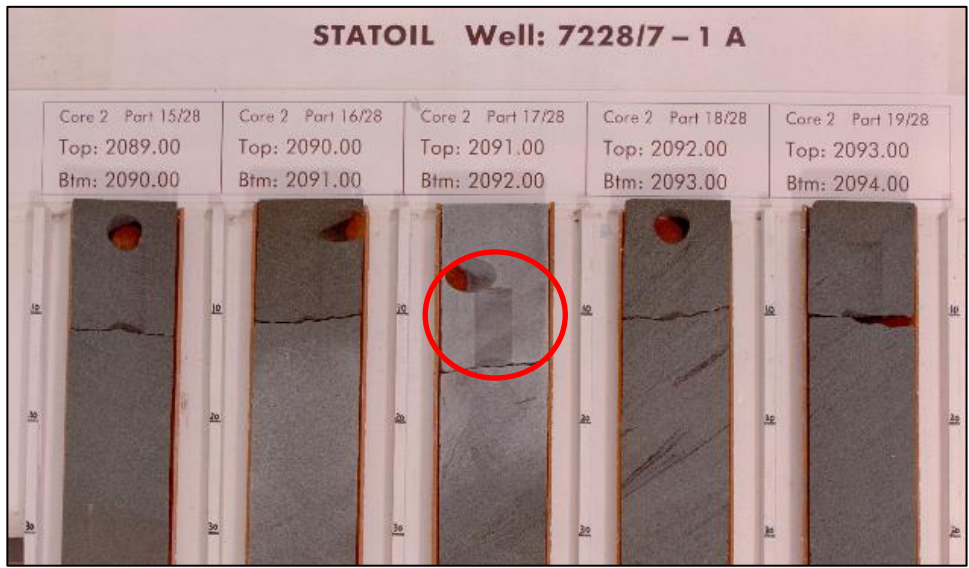
Figure 3: Core photograph for Well 7228/7-1 A for the interval between 2089.0-2094.0 m. Mark the depth 2091.10 m encircled in red from where sample "AB" was recovered (Statoil, www.npd.no )
