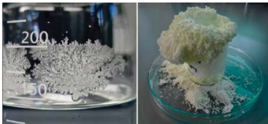
Figure 12. Creeping of a saturated NaCl solution, first as a thin layer of crystals on the side of the beaker (left) followed by secondary creeping on the first structure that formed, leading to a porous mass of crystals (right). [Reprinted with permission from (Bouzig M, Mercury L, Lassin A, Matray JM (2011) Salt precipitation and trapped liquid cavitation in micrometric capillary tubes. Journal of Colloid and Interface Science , Vol. 360, p. 768–776, doi:10.1016/j.jcis.2011.04.095). Copyright (2011) American Chemical Society.]
