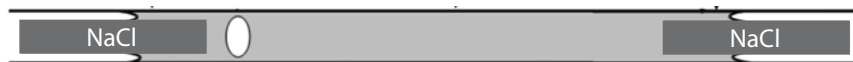
Figure 10. Halite crystals (dark grey), trapping a saturated solution of NaCl (light grey) in which a vapor bubble has formed. Note that the space between the halite crystals and the walls of the capillary is highly exaggerated in order to illustrate the negative curvature of the air–liquid surface. [Modified from Bouzid et al. 2011.]
