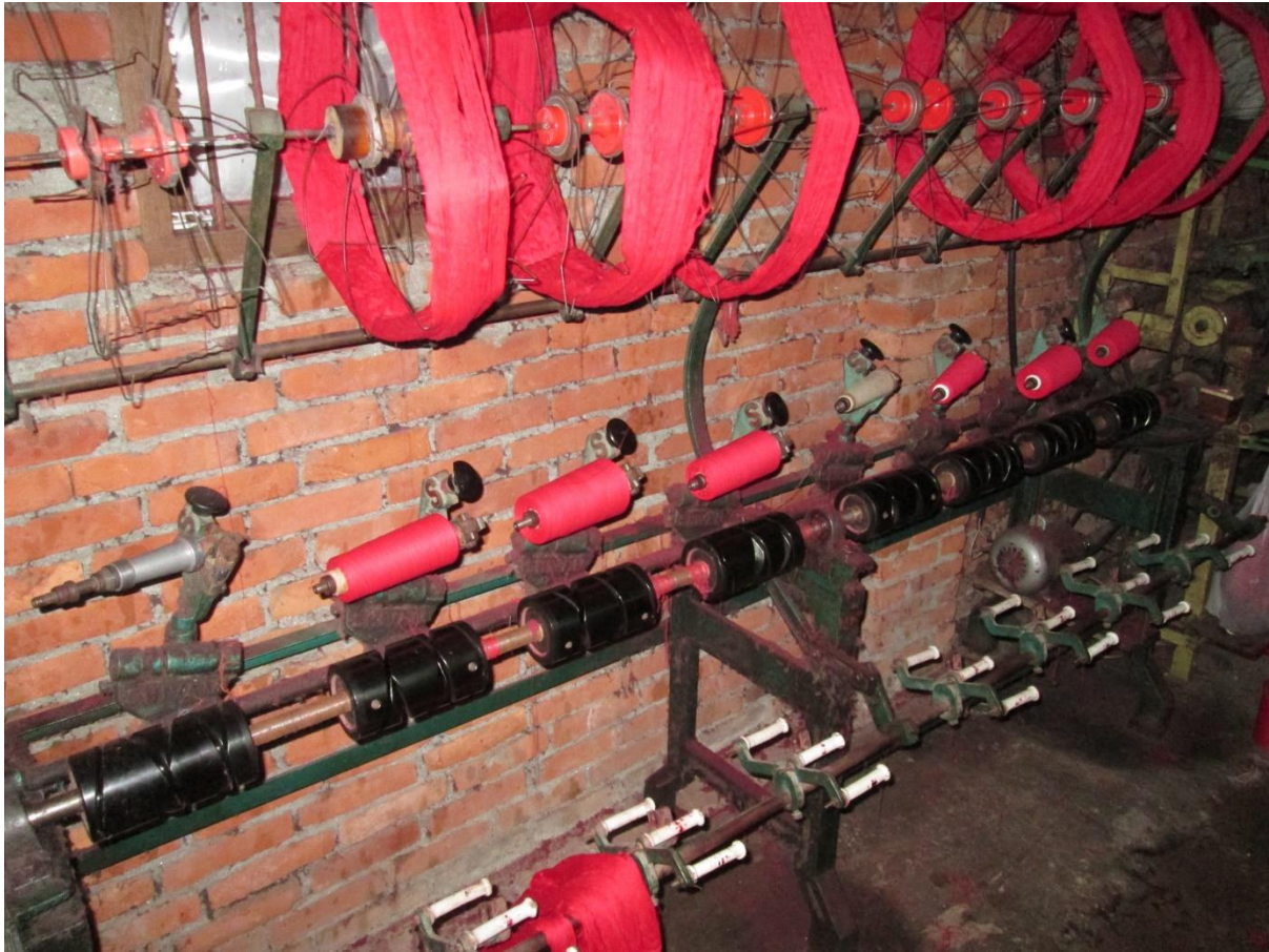
Figure 9: A cone winding system (photo: author)
