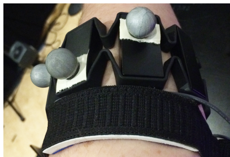
Figure 1: The MYO with three reflective markers, and two BioFlex EMG sensors next to the MYO.
