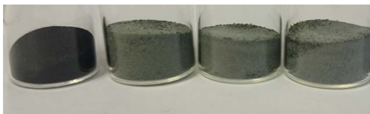
Figure 100. Cat-CoRe-0, Cat-CoRe-5, Cat-CoRe-10 and Cat-CoRe-15 after calcination at 320 °C in air. Sample with lowest rhenium content to the left, and sample with the highest Rh content to the right.
