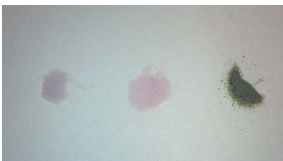
Figure 20. The colours of samples after different steps in the impregnation method; left, after drying of the solvents; middle, before evaporation of the solvents; right, after calcination
