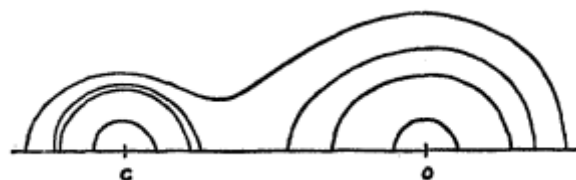
Figure 2. 14: Total electronic density distribution in carbon monoxide. The contours correspond to the values 10.0, 1.0, 0.7, and 0.4, moving out from each nucleus [56].
