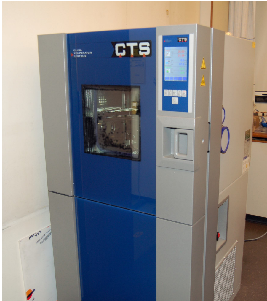
Figure 3.5: CTS-temperature test chamber.
