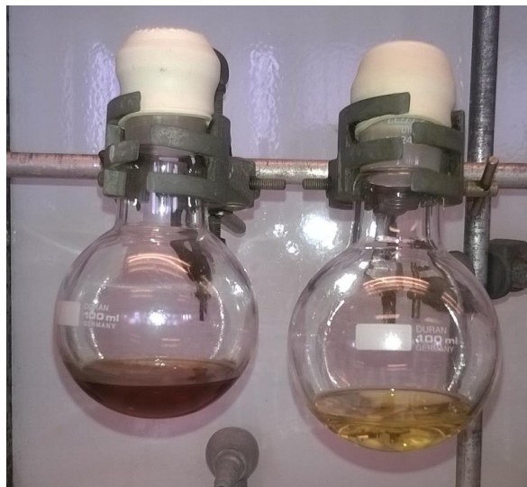
Figure 2.7. Reaction mixtures after 6 days of heating in PhMe. The reaction mixtures were degassed with needles in contact with (left) or above (right) the solution.
