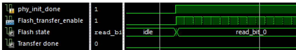
Figure 4.8 - File transfer begins when the DDR3 initialization and calibration is done.
