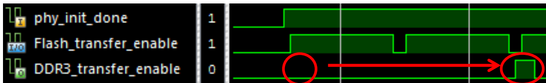
Figure 4.17 - Start-up counter inhibits writing invalid data to DDR3 at the beginning of file transfer.
